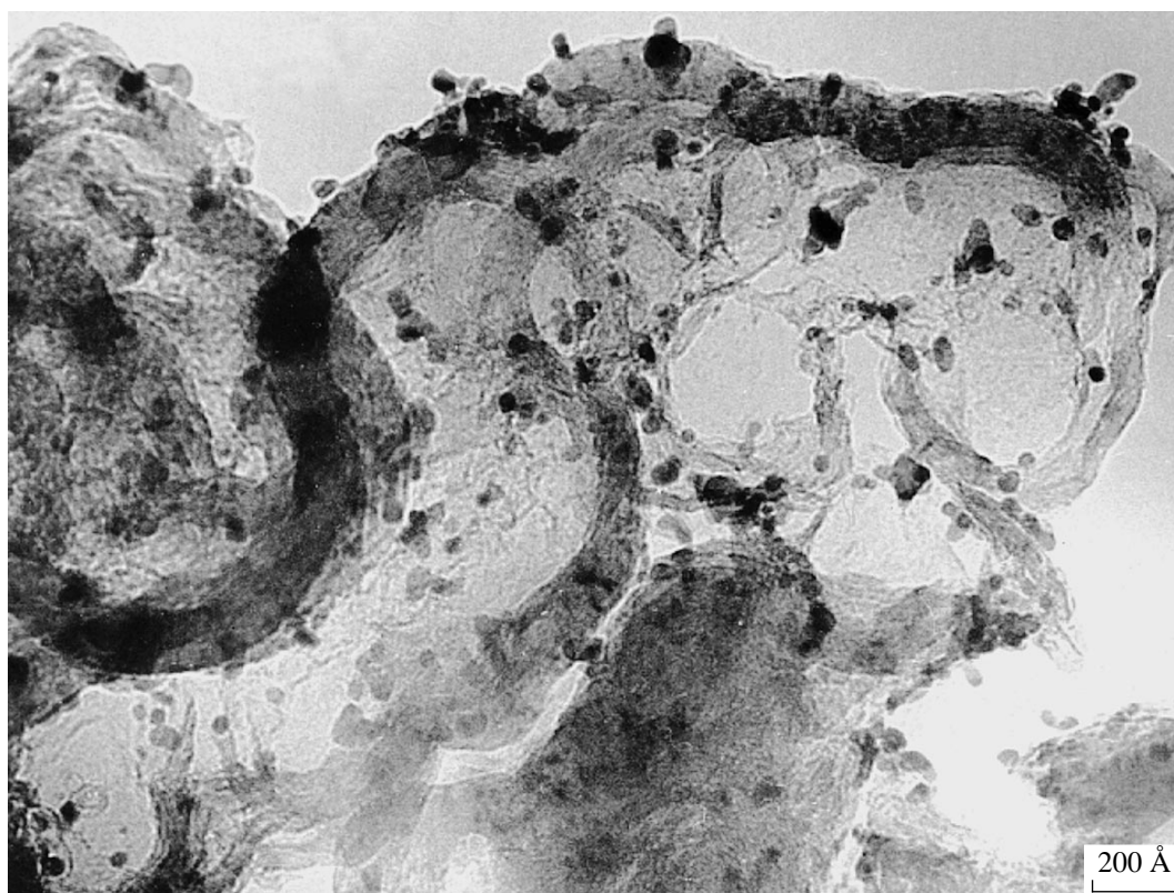
Fig. 4. Electron microscopic pattern of a 4% Pd/Sibunit catalyst prepared from an aqueous sol at [Pd] = 0.01 mol/l and Pd : Mo = 2 .
